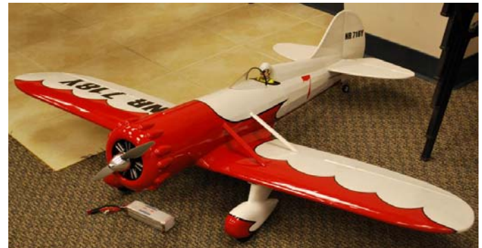
Mark Scherer 's Hobby Lobby electric Gee Bee Senior Sportster ARF. Atlas 28 series motor (46 Size) and a 4 cell Lipo battery.
